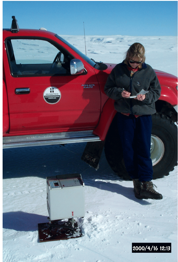
Figure 11. The Scintrex meter levelled on the base station 2023 on Grímsfjall. In 1999 an extension of 1.25 m was added to the hut, making the distance from the hut wall to the point 1.55 m.
