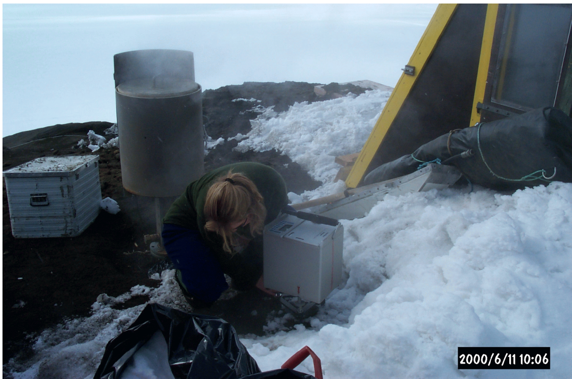
Figure 11. The Scintrex meter levelled on the base station 2023 on Grímsfjall. In 1999 an extension of 1.25 m was added to the hut, making the distance from the hut wall to the point 1.55 m.
