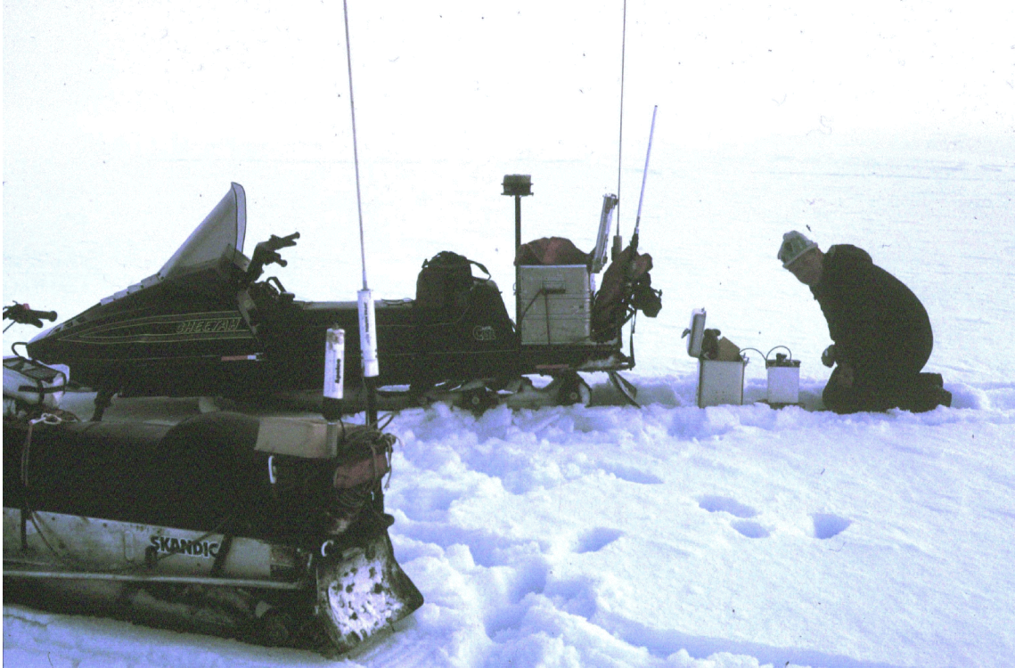
Figure 12. Surveying in Grímsvötn in 1988. Loran-C antennas are mounted on the snowmobiles.
