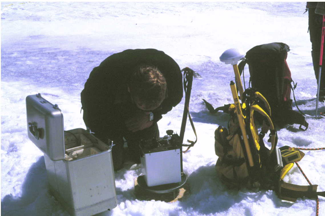
Figure 13. Surveying in Gjálp in 1997. The LaCoste meter is placed on a wooden plate. Positioning and elevation measurements done with the Trimble DGPS receiver.
